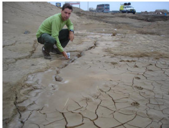
Fig. 11. Large sand cone with possibly liquefied fine grains.
