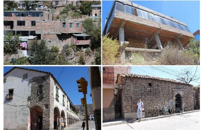
Fig. 13. Typical buildings that present a certain seismic vulnerability level in Ayacucho city.
